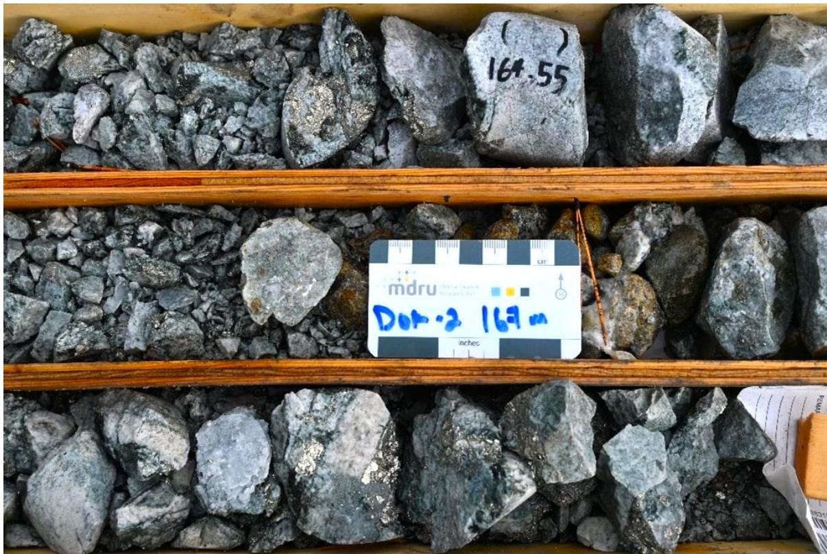
*Figure 5 – Intense phyllitic alteration with pyritic stockwork from DOK2023-02*
