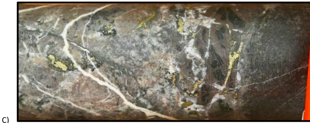
Figure 2 – select core intervals from first hole showing chalcopyrite mineralization.
