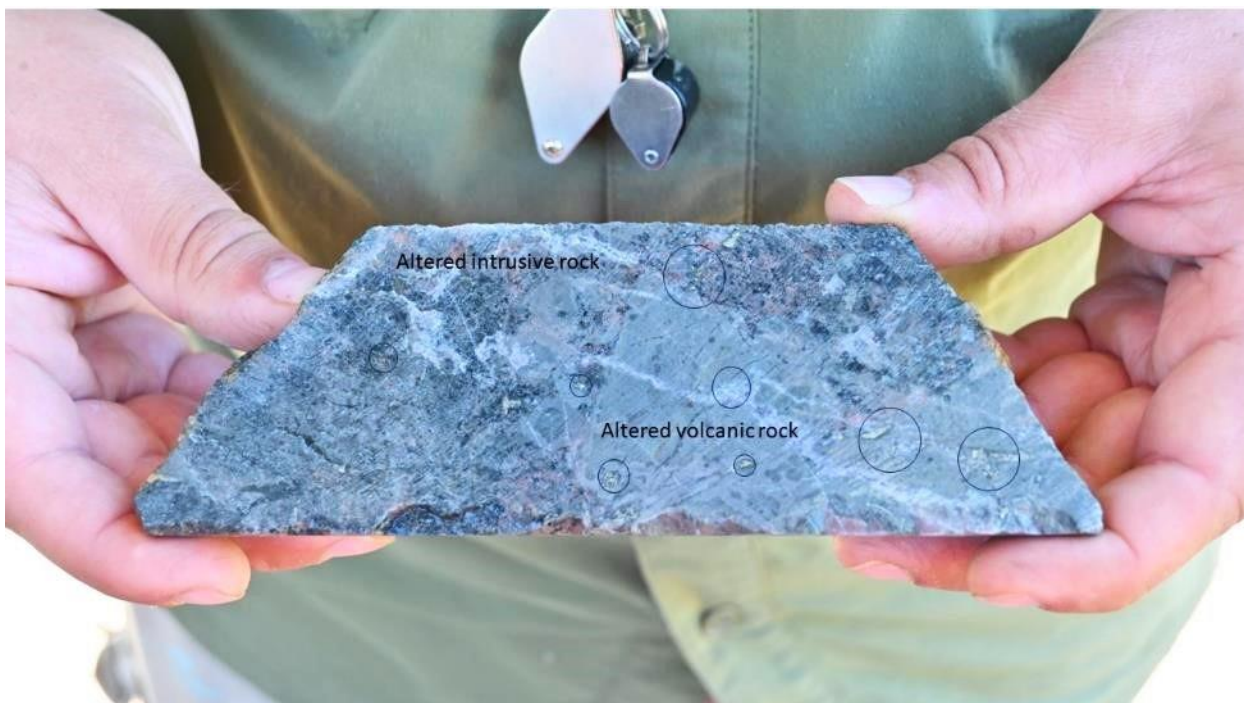
Figure 1: Sample from DK2023-001 showing breccia texture comprised of intrusive and volcanic rocks. Black circles highlight chalcopyrite.
