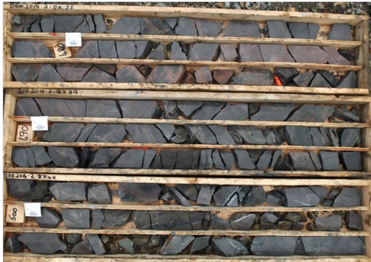
Core from Dok 2014-2: porphyry-style alteration and mineralization.
