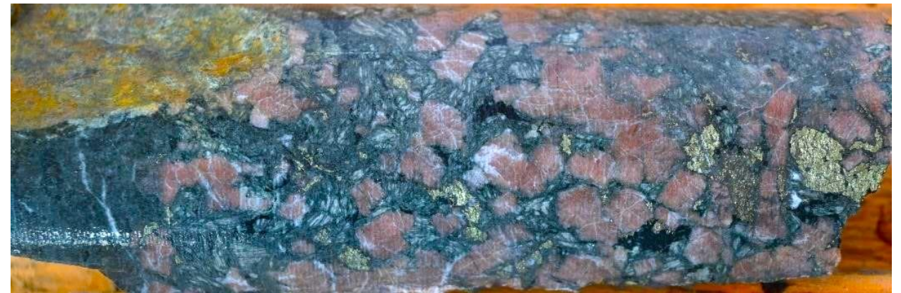
Potassic alteration with chalcopyrite mineralization in hole Dok2023-03
