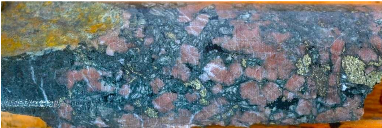
Potassic alteration with chalcopyrite mineralization in hole DK-2023-03
